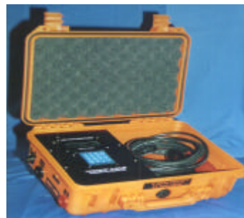
Figure No. 4 GPS Synchronised Current Interrupter
