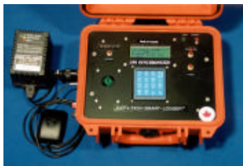
Figure No. 7 GPS Synchronized Data Logger
